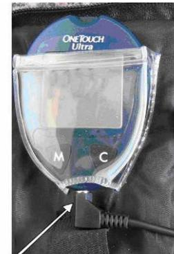
Plug in jack and press firmly into place
