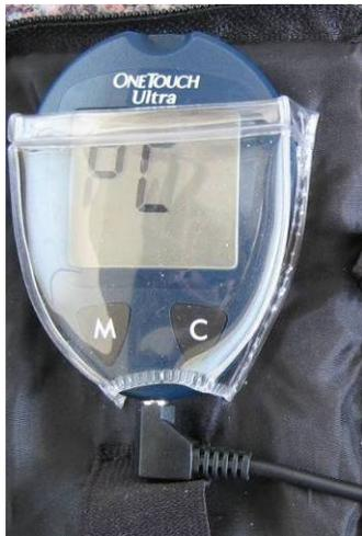
**Figure 4: PC shows on the OneTouch Ultra when the GMA is receiving your readings.**
