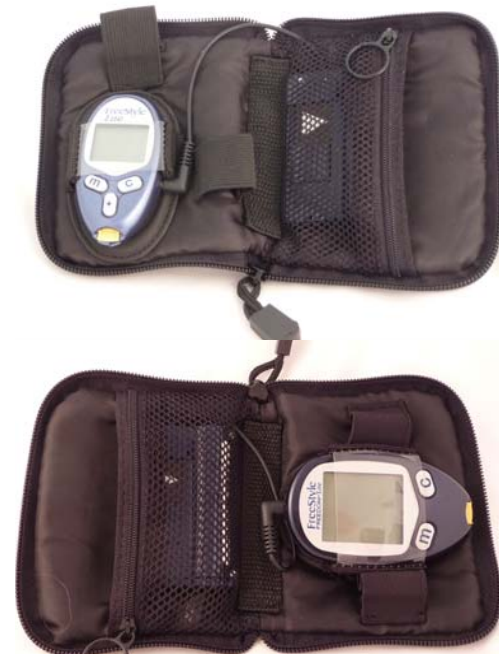
Figure 5: glucose meter and GMA in carrying case. Above: FreeStyle Lite and FreeStyle Freedom Lite. Note different position of GMA to make closing cover easier with larger meter
