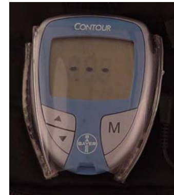
Figure 6 “---“ shows on the glucose meter when the GMA is receiving your readings.
