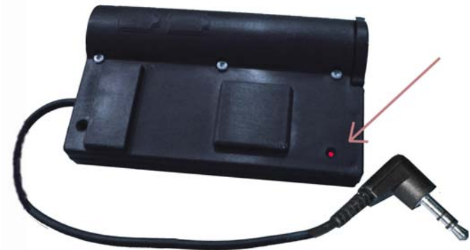
Figure 1: Red light indicates status of the GMA
