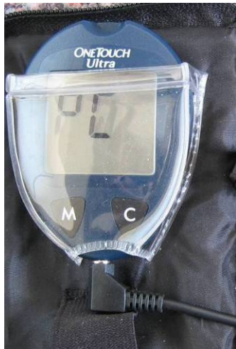
Figure 4: PC shows on the glucose meter when the GMA is receiving your readings.
